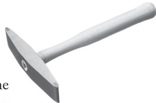
Mill Pick is handy for chiseling lines into stone or dressing edges. While the Mill Pick can also be used for light trimming of thin stone, the over-swinging required to shape thick pieces of hard stone can result in a broken handle.
