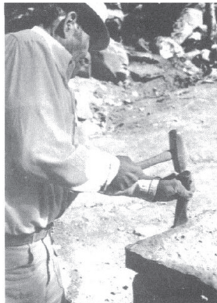
A pitching chisel is used to remove unwanted material in a hurry. Here Soto uses one to clean up a ragged edge on a flagstone.
