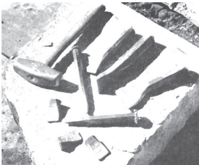
Clockwise from top: Soto's hammer, a point, two pitching tools, a toothed chisel and a lifter. The three wedges were custom made by a blacksmith.
